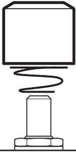
A fine spring is provided for each single & upper knob, in order to maintain electrical contact with the knob.
